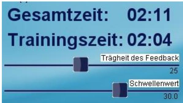
The **total time (Gesamtzeit)** provides information about the length of the session, while the **training time (Trainingszeit)** tells how long the user has exceeded the desired **threshold (Schwellenwert)** value, concerning temperature. In this case the adjusted value is 30° Celsius which means that the training time starts counting, when the temperature has exceeded 30° Celsius and stops right away if the temperature falls below this value.
