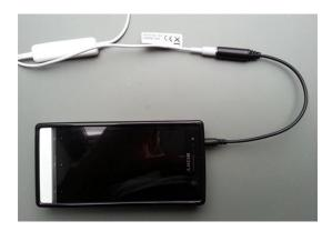
Adapter cable inverts connector pins of microphone jack – only for use with certain Android devices!
